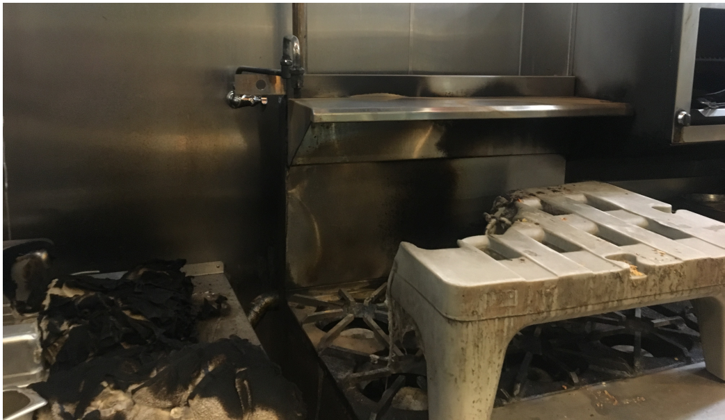
Burnt rags [left] and melted step stool [right] on top of gas burner range.
